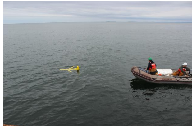
Deploying one of the two Slocum Gliders
