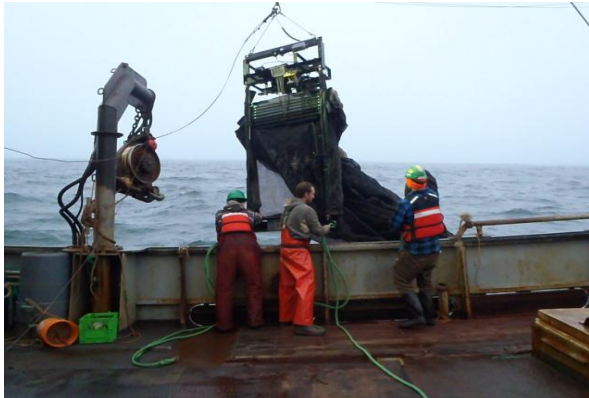
MOCNESS multiple net plankton collection device
